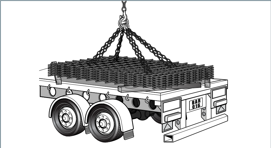
Lift from all corners with chains positioned as indicated. The legs of the chains should be of adequate length to permit an acceptable chain angle as detailed in the site lifting plan.
